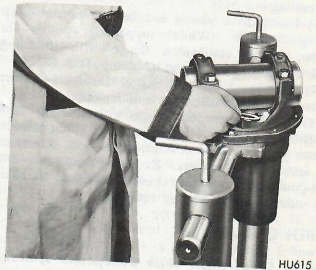
Fig. 29 Determining Spacer Thickness
