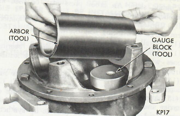
Fig. 28 Installing Arbor in Carrier
